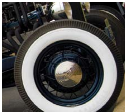
The popularity of white sidewalls in the US market presents problems due to PPD staining
